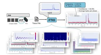
FTIO in a Nutshell. The I/O requests are captured using TMIO and analyzed using FTIO to obtain the frequency of the I/O phases alongside the confidence in the results.
